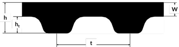
HY-Profil - Geometry data based on ISO ISO 13050 [Profile system H]
